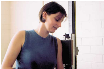
Measuring push with the shoulder at 90% of shoulder height
