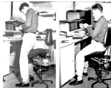
Using the seat at this height the mechanic can sit, or stand, at the bench with ease. The seat shown is a development versus that sits to the required angle automatically as the seat is raised.
