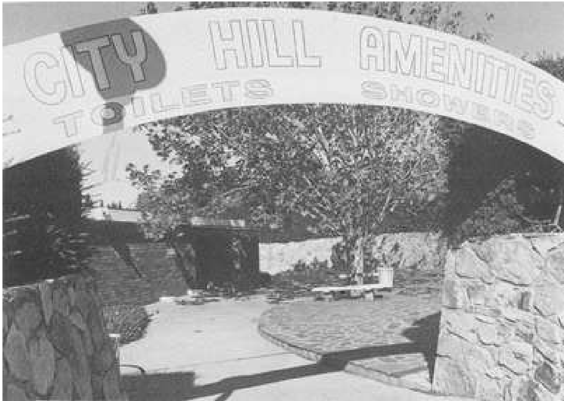
This women's lavatory is an example of poor design. It is badly lit and surrounded by high walls and hedges, making surveillance by passers-by impossible. Photographer Marie Colvill, Science Photography Unit, ANUPS, Australian National University
