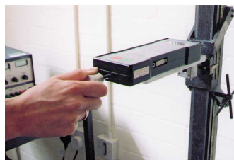
Measuring twist force on the 20 mm knob
