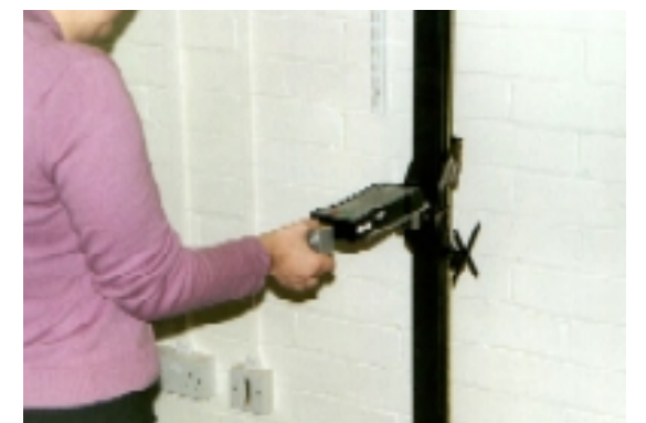
Experimental trial: Chuck pinch-pull (20mm block)
